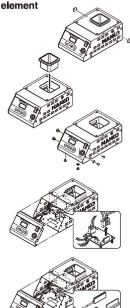
Loosen the screws on both sides of the unit.
